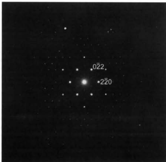
Fig. 2. Electron diffraction pattern of the C 60 low-temperature phase with the incident beam parallel to the \langle 111 \rangle direction. It shows sixfold rotational symmetry corresponding to the space group Pa\bar{3} . In the center of the triangles of intense spots near the center beam there are some weak spots arising from planar disorder, such as stacking faults on the (111) plane, which cause reciprocal lattice nodes of the upper zone such as the 111 reflection to be streaked (Ishiguro & Hirotsu, 1992).
